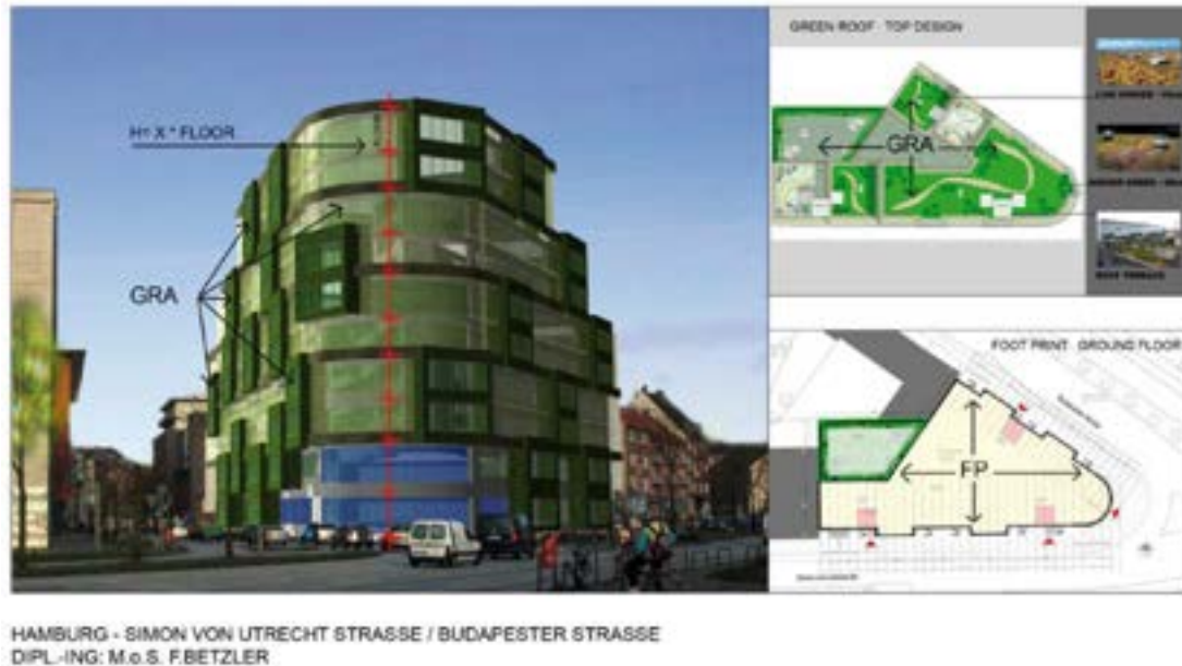
Fig. 1 Illustration of different greening parameters used to calculate the Green Density Factor (GDF), see list below for details. The footprint of the building is marked as FP, the green façade areas as GFA, and the green roof area as GRA.
